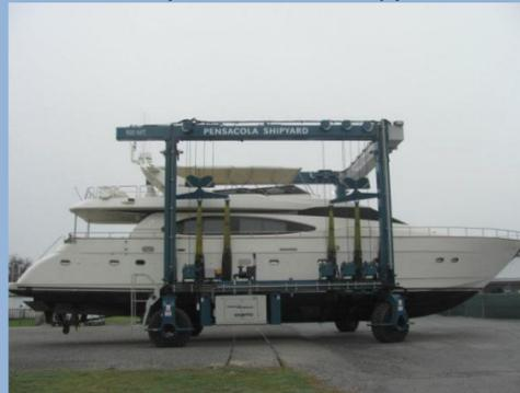
An 85' Azimut heads to the pressure wash pad before being placed in the yard.
