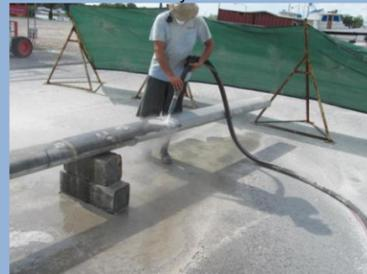
Removing paint from an aluminum mast
