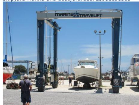
Centering the lift over a vessel
