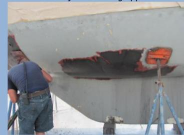
Removing the bottom paint and leaving the barrier coat
